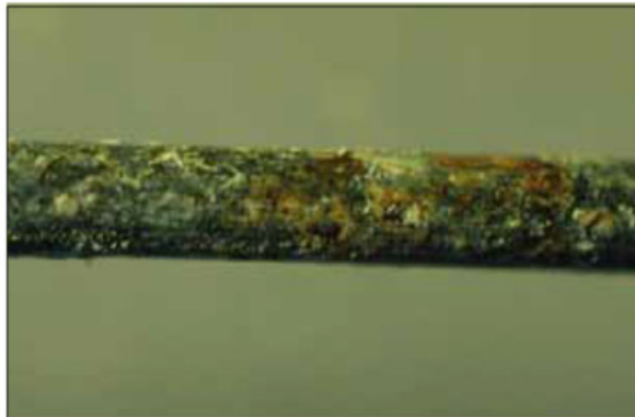
The rust occurrence for 1mm zinc galvanized wire after 200hours
